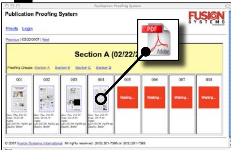
The Publication Proofing System dynamically posts JPEG page images that are linked to halftone-dot PDFs to deliver 'Dot-Locked' accurate digital proofs. Pages are automatically displayed by publication, and section, as pages are processed.
